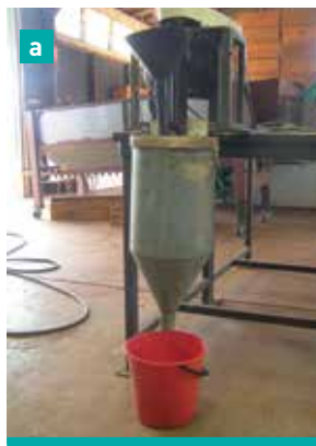
Fig. 23a, b: A mechanised rotary sander houses a spinning sandpaper disc (b) to scarify seed.
