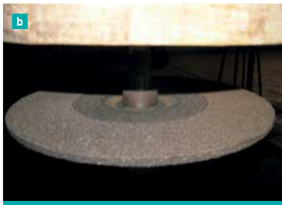
Fig. 23a, b: A mechanised rotary sander houses a spinning sandpaper disc (b) to scarify seed.
