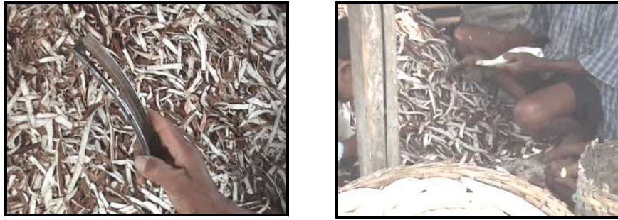
Figure 1. A special knife made from bicycle wheel steel used for peeling cassava roots in home-scale cassava starch factories
